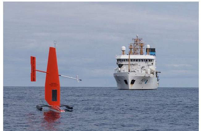
Figure 2. Saildrones—autonomous sailing vessels with customized acoustic technologies— can be used to study whales, fish, and seals in remote parts of the ocean.
