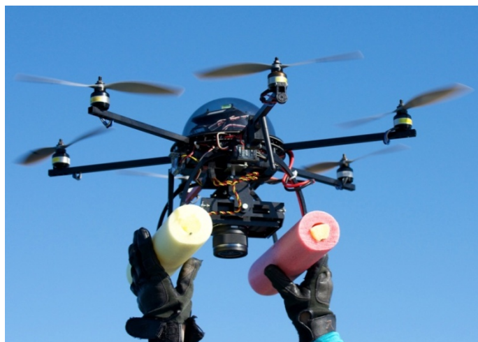
APH-22 hexacopter with gimballed camera for photogrammetry being hand-launched (J. Durban, H. Fearnbach, SWFSC)
