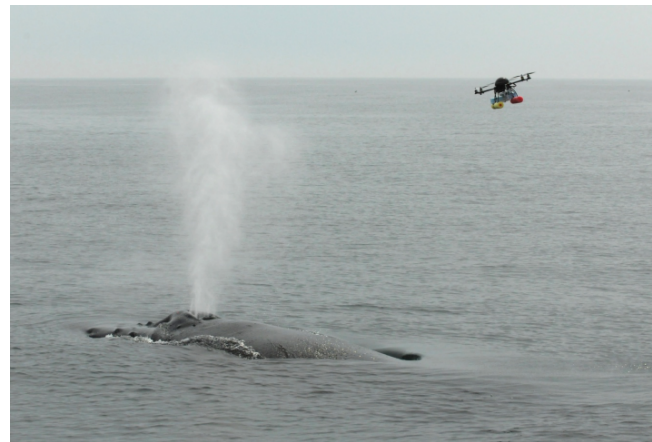
APH-22 hexacopter maneuvering to collect an EBC sample from a humpback whale off Cape Cod. (J. Durban, H. Fearnbach, SWFSC; in collaboration with M. Moore, Woods Hole Oceanographic Institution; NMFS Permit # 17355).
